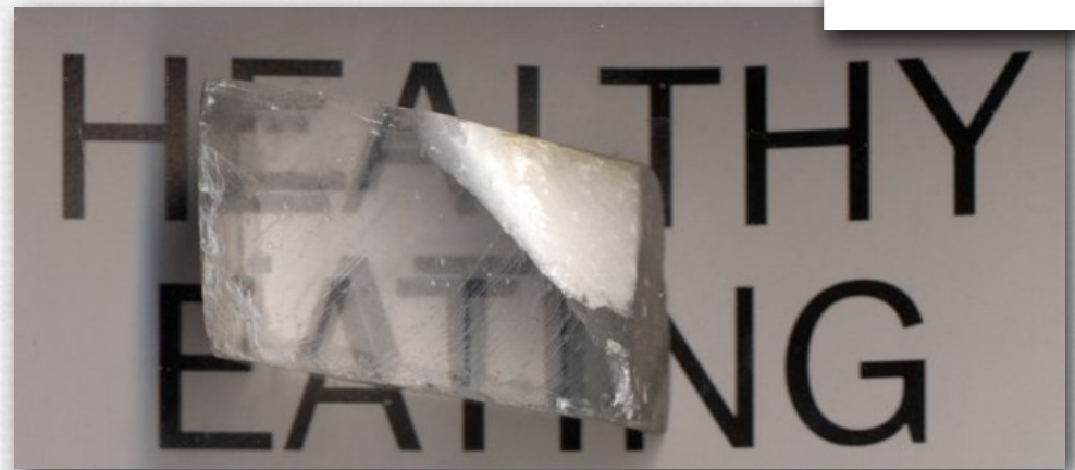
birefringence in a calcite crystal
