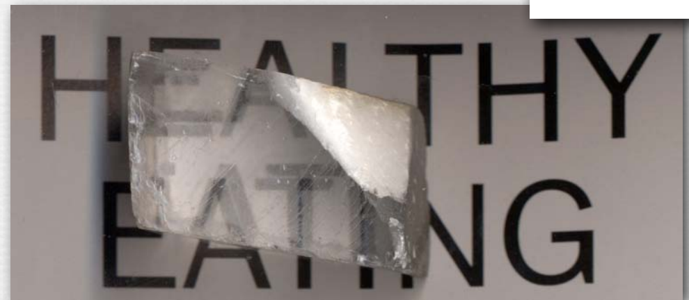
birefringence in a calcite crystal
