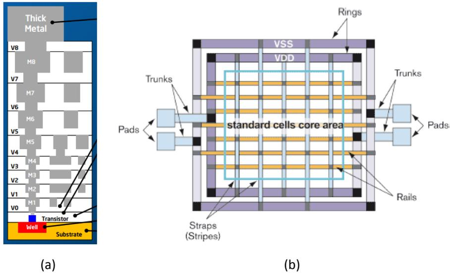
Figure 2. (a) metal layer structure of Intel 32nm RF technology. (b) Schematic of power and ground mesh network [2].
