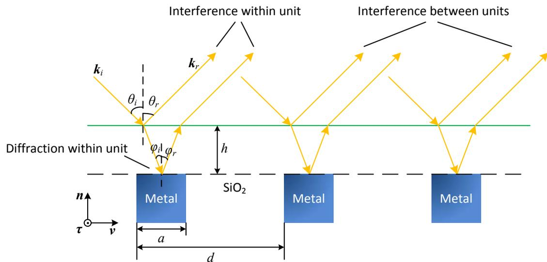
Figure 5. Various optical effects on wafer surface
