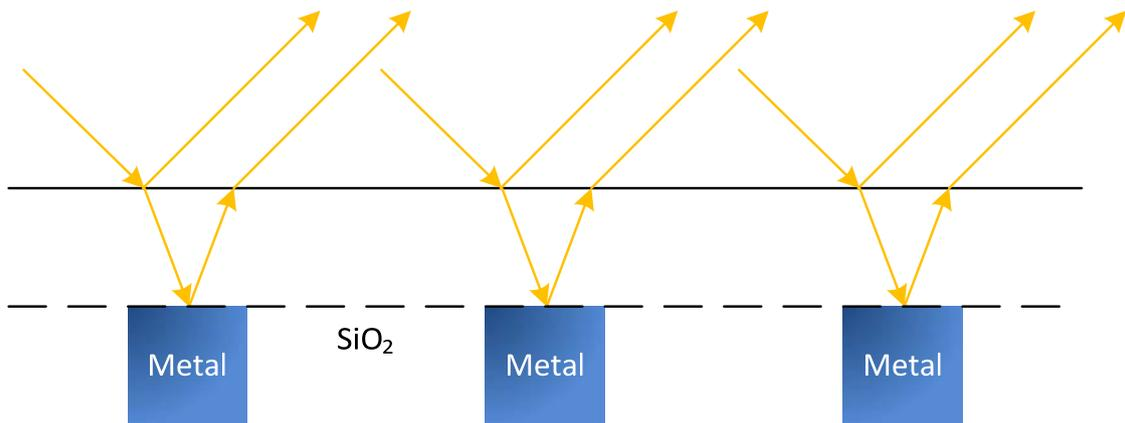
Figure 3. Simplified structure of the wafer surface
