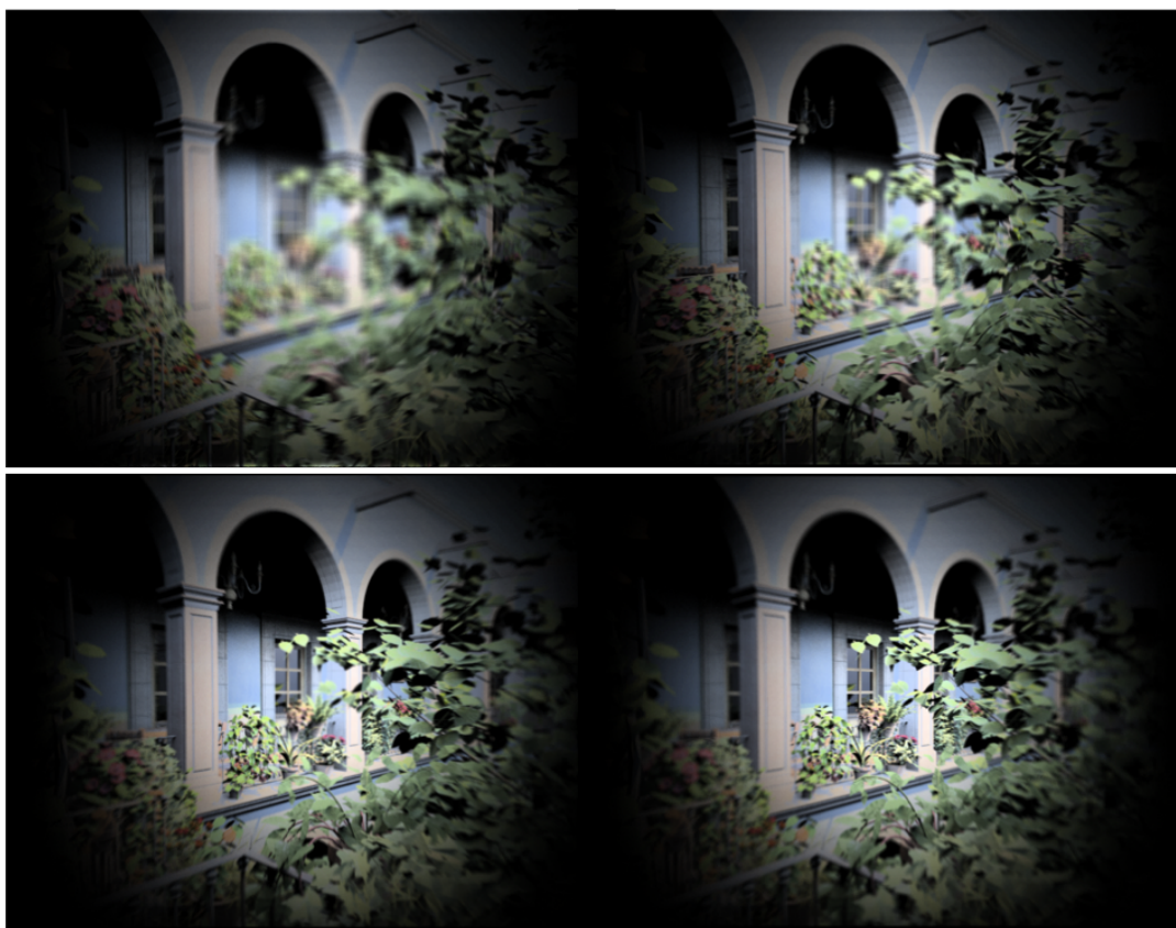
Figure 11: San Miguel scene focused at different depth using a single spherical main lens. Note on the top row, how the foliage at the periphery of the main lens got focused earlier than the center part. This is caused by the spherical lens aberration that focuses light at the periphery at a closer distance than the actual focal length.
