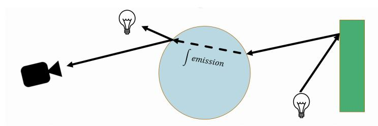
In my prototype of **VolumeLight**, the integration over the emissive volume is done using a midpoint-method numerical integral approximation; the line segment used is chosen using the point of intersection with the sampling ray and the refracted direction it takes within the surface.
