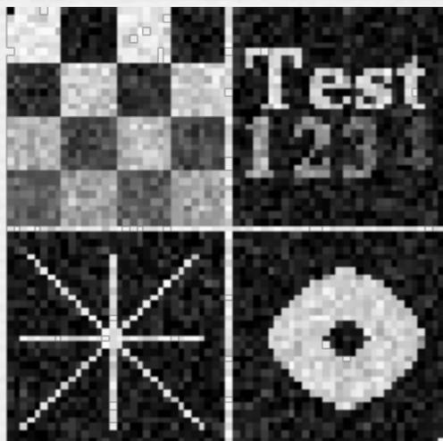
Test image with AWGN (additive White Gaussian Noise)
