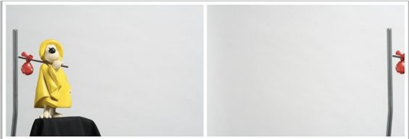
Figure 3. Configuration to reveal the presence or absence of parallax. The subject is first placed at the left side of the frame, and subsequently at the right side after rotation of the camera about a vertical axis with the help of a panoramic tripod head.
