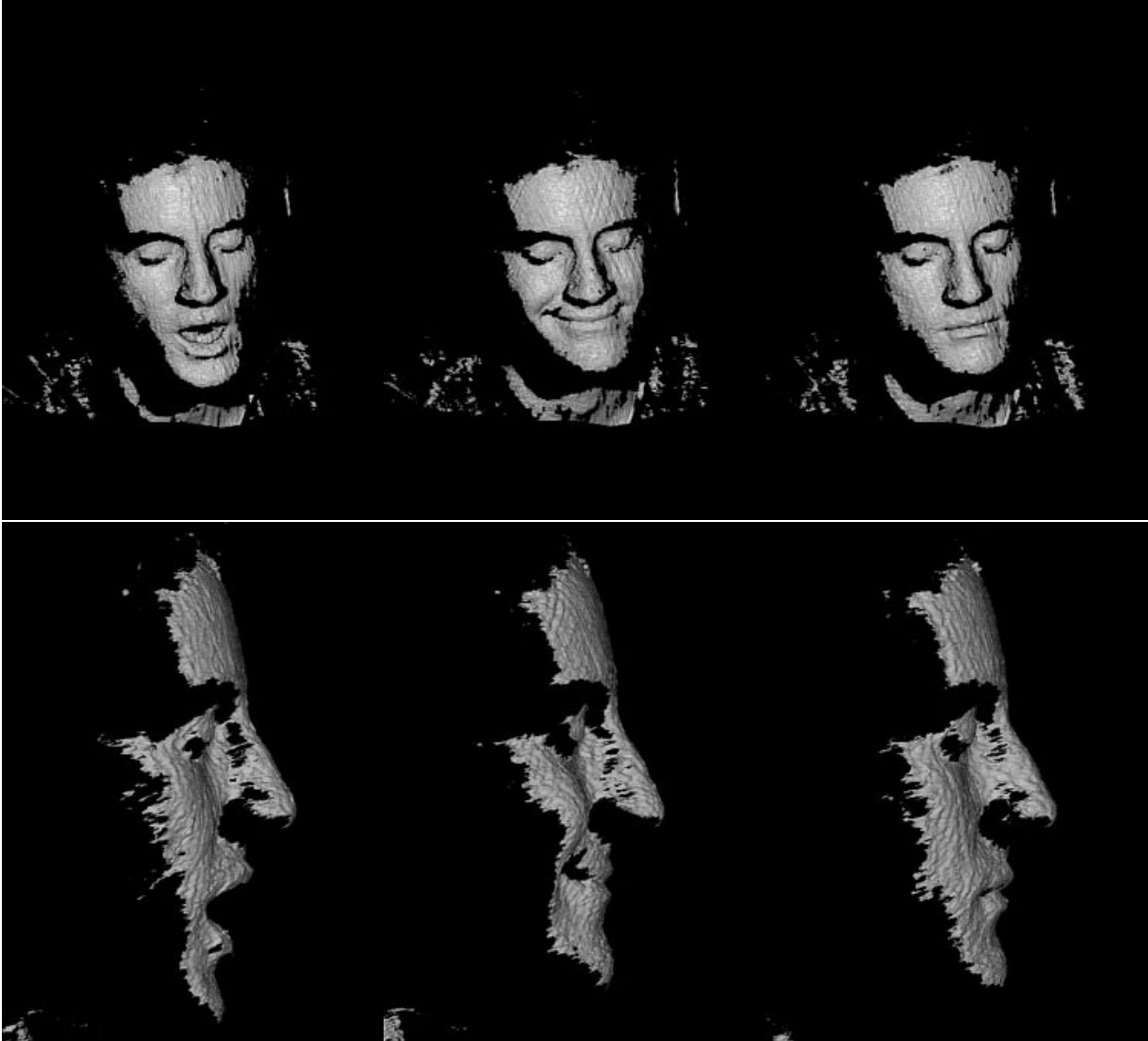
Figure 18: Depth estimates on a dynamic scene (one of the authors smiling), captured at 40 Hz. We show two views (frontal on top and side on bottom), for three instants in time. Note recovery of subtle features like the cheek deformation. Spacetime stereo provides a new way of recovering depth in dynamic scenes, which has been difficult for previous algorithms.
