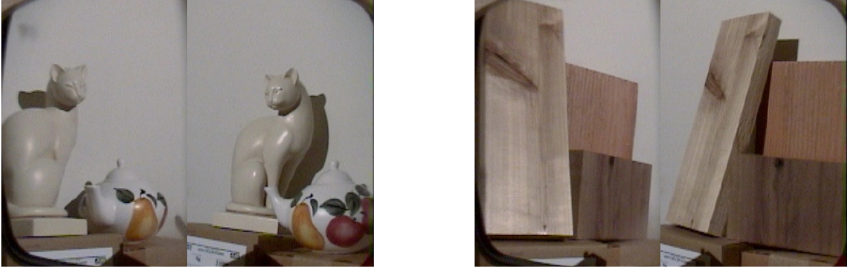
Figure 9: Sample stereo pairs for the two scenes used in our experiments. Note the specularities on the cat sculpture and the regions of uniform texture on the wood blocks, both of which make traditional spatial stereo matching difficult.
