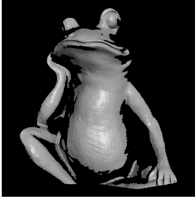
Figure 15: Estimated depth using temporal stereo when the object is static
