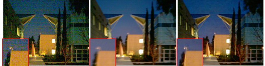
Figure 11: Low-Light Imaging. We use the FCam API to create a low-light camera mode. For viewfinding, we implement the method of [Adams et al. 2008] which aligns and averages viewfinder frames. For capture, we implement the method of Tico and Pulli [2009], which fuses the crisp edges of a short-exposure high-gain frame (left), with the superior colors and low noise of a long-exposure low-gain frame (middle). The result is fused directly on the camera for immediate review.
