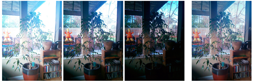
Figure 10: HDR Imaging. A programmable camera running the FCam API improves HDR acquisition in three ways. First, it lets us cycle the image sensor through three exposure times at video rate to meter for HDR and display an HDR viewfinder. Second, it lets us capture the burst of full-resolution images at maximum sensor rate to minimize motion artifacts (the three images on the left). Finally, the programmability of the platform lets us composite and produce the result on the camera for immediate review (on the far right).
