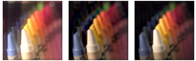
Figure 13: Aliasing reduction by superior filtering. Rolloff correction is applied. Left: Quadrilinear filter (width 2). Middle: Kaiser-Bessel filter, width 1.5. Right: Kaiser-Bessel filter, width 2.5.
