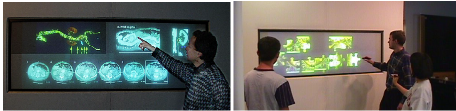
Fig. 1. A large tiled display on which multiple users can interact using laser pointers.
