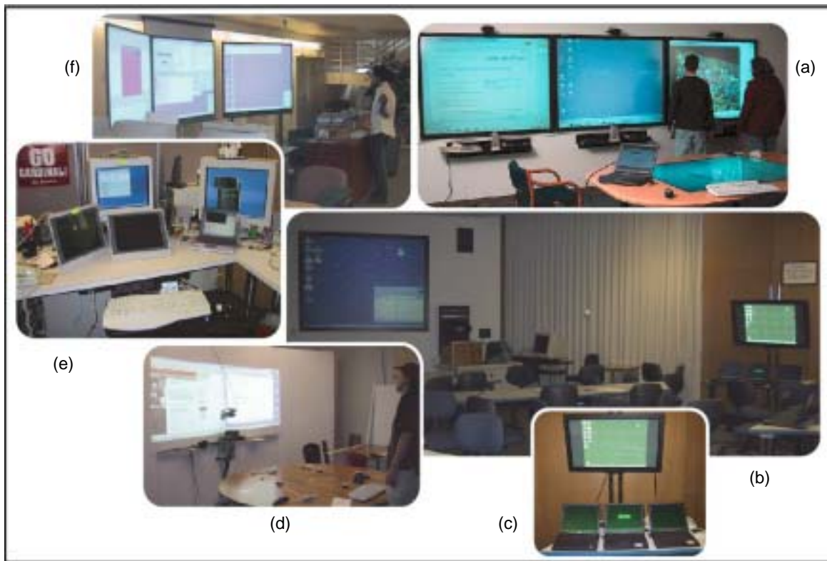
Figure 3. PointRight configurations, clockwise from the top right. (a) The iRoom, with its three rear-projected SMART boards and table. The free-space wireless mouse and keyboard, along with a laptop, are shown on the table. (b) The Writing Laboratory, with its big front display and one of its 5 plasma displays. (c) Close-up of the plasma display and its three laptops. (d) Project learning lab, two projectors pointed at a foam core screen, controlled by a wireless mouse and keyboard. (e) A desktop iRoom. (f) The iRoom used for construction management, with its three front-projected, touch sensitive SMART boards. The free space wireless keyboard and mouse are placed behind the projectors to eliminate shadowing.
