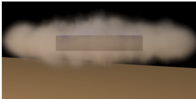
Figure 6: Two stills from the rotor animation. A box is rotating inside the smoke causing it to disperse. Notice how the smoke is sucked in vertically towards the box as it is pushed outwards horizontally. The simulation time for a 120x60x120 grid was roughly 60 seconds/frame.
