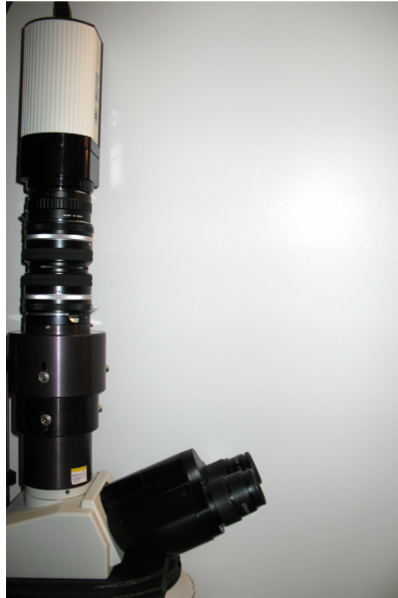
Figure 1.5: The finished light field microscope built on top of the Eclipse 80i. The camera (Retiga 4000R) is connected to the back end of a Nikon 50mm f/1.4 lens. This lens's front is connected to the front of another Nikon 50mm f/1.4 lens using a nose-to-nose filter ring adapter. The back side of the second Nikon 50mm f/1.4 lens is connected to the microlens array holder. Finally, the microlens array holder is attached to the top of the camera port of the universal epi-illuminator.
