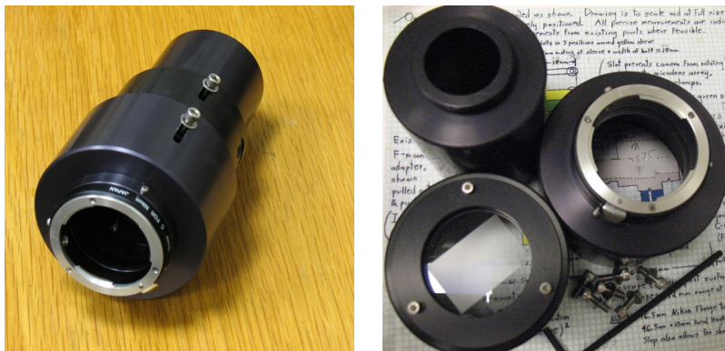
Figure 1.4: The finished, assembled microlens array holder is shown in (a). The three pieces are shown separately in (b), with a microlens mounted.
