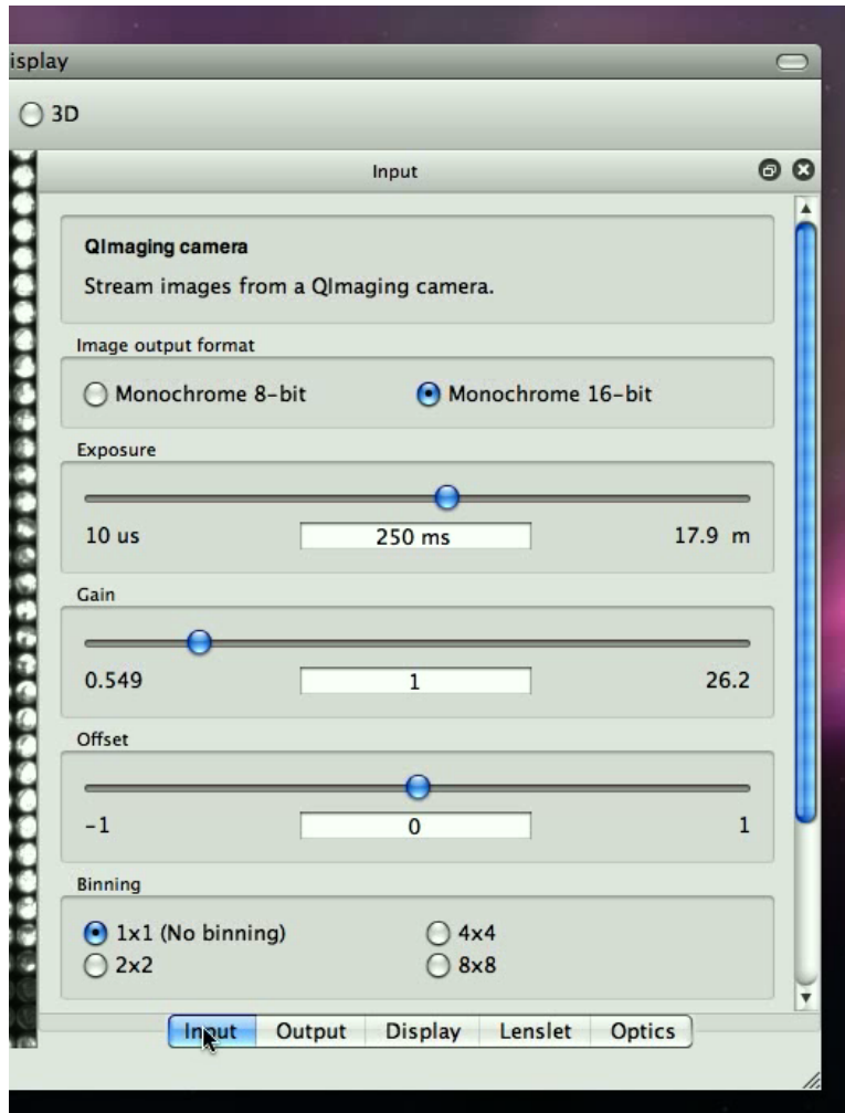
Figure 2.3: This is the input panel for controlling camera settings. The exposure slider is the most important; gain and offset should be left at 1.0 and 0.0 if possible. You can scroll down to see some information about the current camera.
