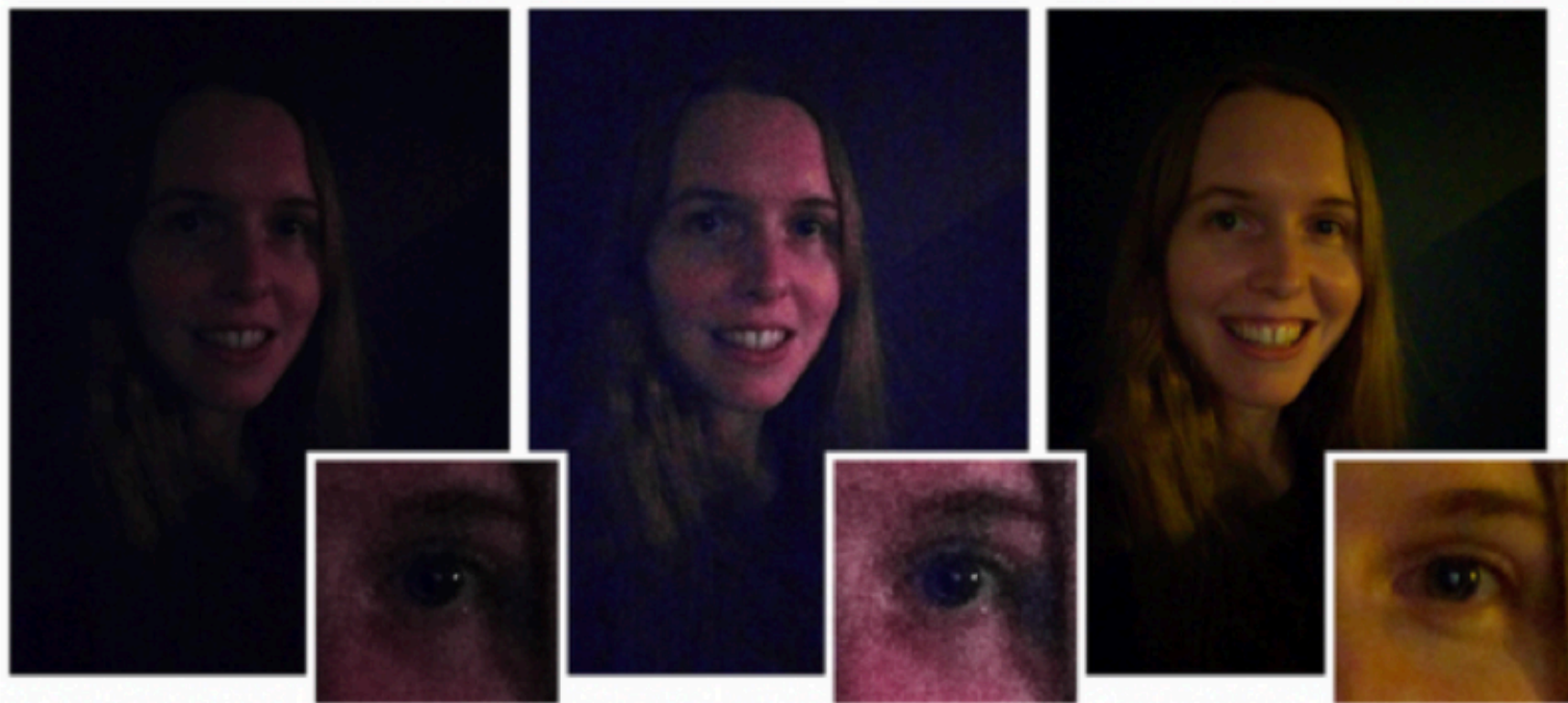
Figure 1: A comparison of a conventional camera pipeline (left, middle) and our burst photography pipeline (right) running on the same cell-phone camera. In this low-light setting (about 0.7 lux), the conventional camera pipeline underexposes (left). Brightening the image (middle) reveals heavy spatial denoising, which results in loss of detail and an unpleasantly blotchy appearance. Fusing a burst of images increases the signal-to-noise ratio, making aggressive spatial denoising unnecessary. We encourage the reader to zoom in. While our pipeline
