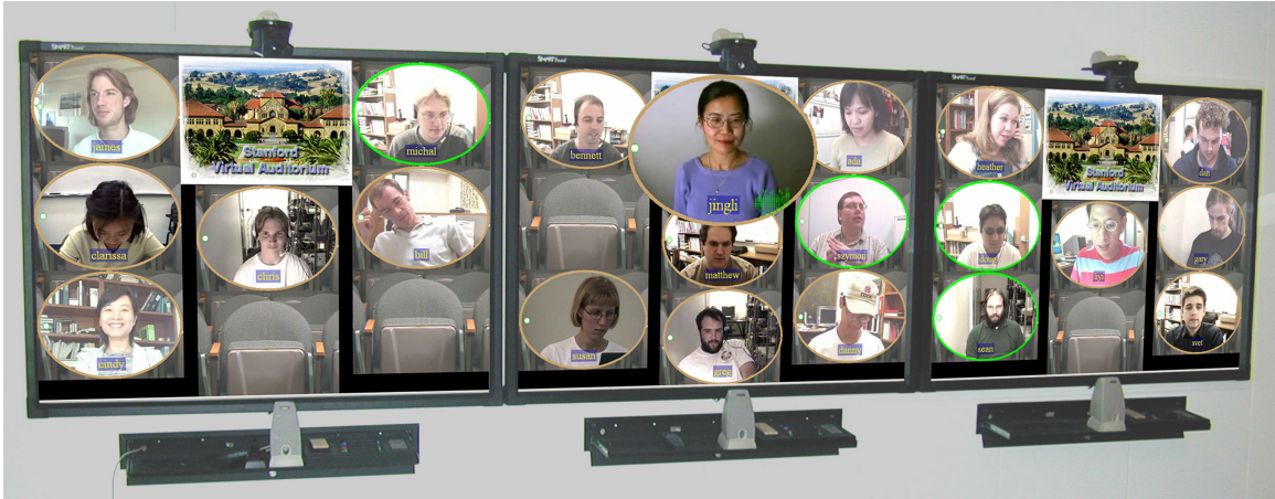
Figure 6.1. The Video Auditorium display wall. This wall can display 24 students and the instructor can move students to different seats. Videos are elliptically shaped to provide a common background for all students. A student's voice is rendered from the loudspeaker closest to his image and his instantaneous audio amplitude is displayed next to his name. The audio localization and amplitude display allow the instructor to easily identify the speaker. Directly below the cameras are regions called the visual teleprompters that show visual aids or students in directed gaze mode.
