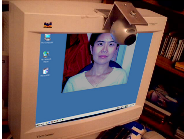
Figure 5.7 Desktop videoconference prototype. We constructed a mechanical camera holder for supporting eye contact in a desktop video communication system.
